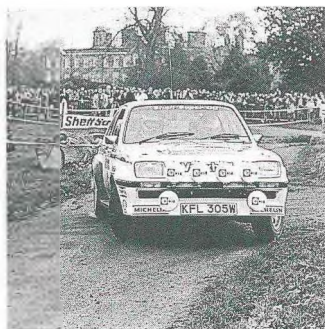
During 1980 Vauxhall produced the Chevette HSR, an 'Evolution' of the 2300HS, complete with wheel arch extensions, plastic sills, and revised rear axle location. This was Tony Pond's DTV 'works' car on the Lombard-RAC rally of 1981.
